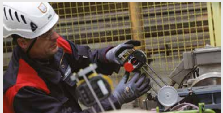
Laser-optical alignment of an installed cardan shaft
