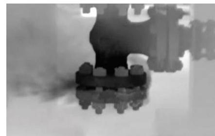
*Figure 2: OGI allows users to spot the source of leaks, such as in this valve.*
